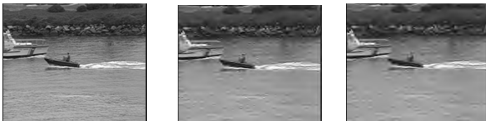
Figure 1. Frame 32 of QCIF “Coastguard” video sequence. Left: Original frame; Middle: SelectFocusVIDEO at 13 kilobits/second and 3 frames/second; Right: SelectFocusVIDEO at 10 kilobits/second and 3 frames/second.
